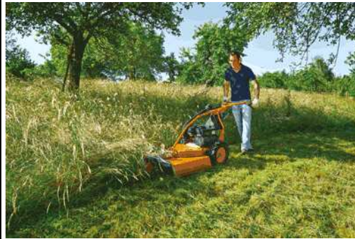
Picture 2: The high grass mower: It has to cope with a lot of "material" and therefore usually has a simple side discharge or, even better, a rear discharge with closed mowing hood.
