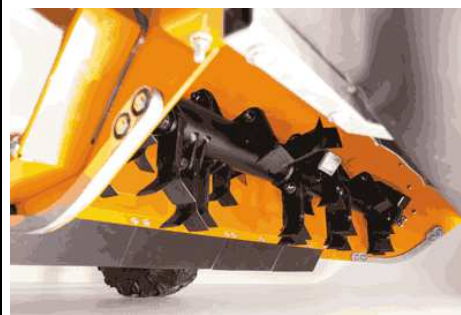
Picture 4: The flail mower: If the flails hit a foreign object, they can fold away - a decisive advantage compared to the sickle mower.
