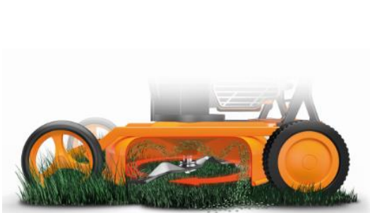
Figure 3: In the mulching bell, the rotating blade generates an air stream that swirls cut grass. The grass is finely shredded by a special mulching blade and returned to the surface of the lawn.
