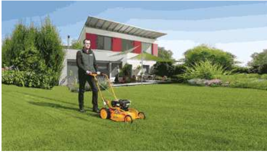
Figure 1: Mulch mowers can be recognized by the lack of a collection bag and the mowing hood's round, closed shape.
